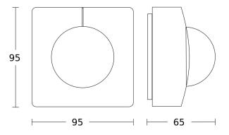
Possible mounting height: 4,00 m – 16,00 m Orange: radial and tangential
